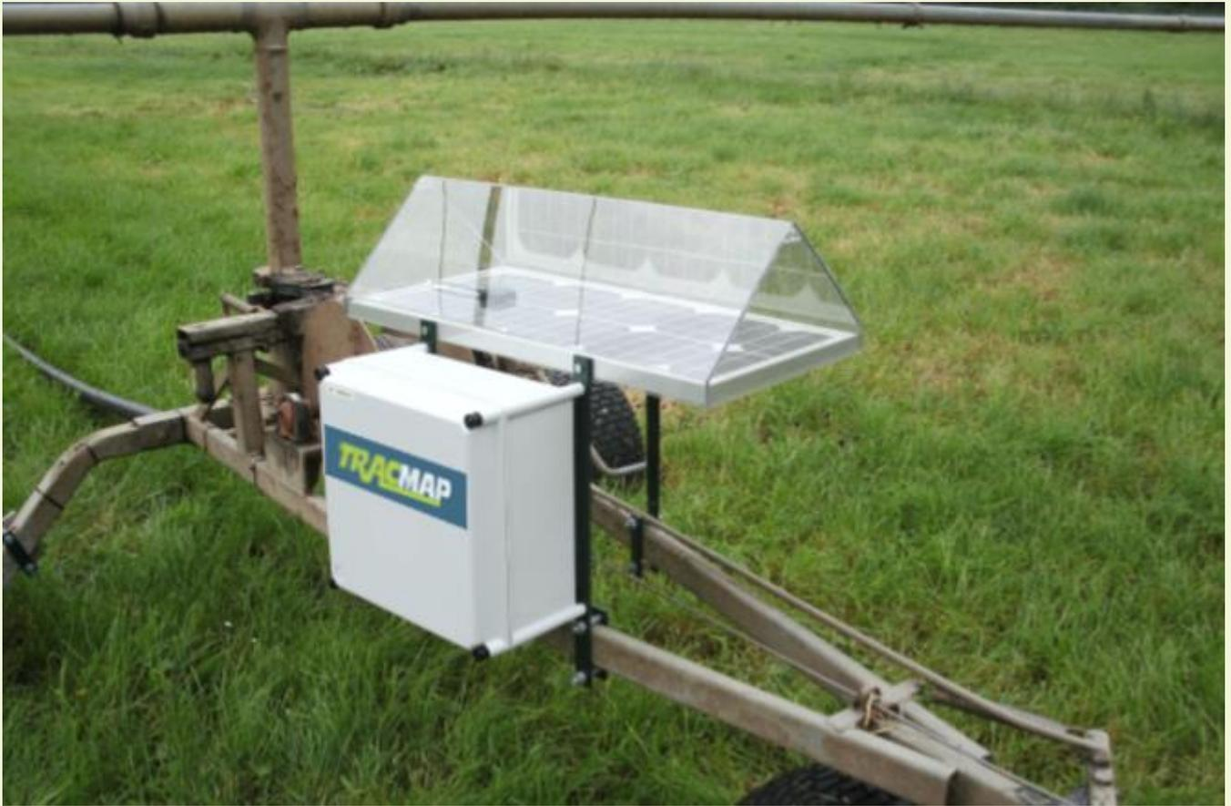
Picture 1: Typical Irrigator Monitor Installation
