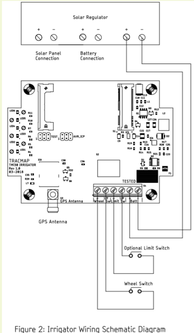
Figure 2: Irrigator Wiring Schematic Diagram
